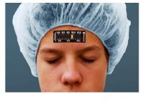
Liquid crystals that change color with changes in temperature are known as Thermochromic Liquid Crystals (TLCs). Scientifically they are identified as Cholesteric Liquid Crystals. Micro-encapsulation is the process that primarily protects, stabilizes and makes the liquid easier to use.
